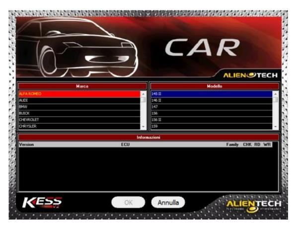
The window with every kind of vehicle displays: brand, model and the version of the ECU related to the engine equipped on the vehicle. On the right side there are three checkboxes that indicate what KESSV2 can do: Checksum (CHK), Reading (RD), Writing (WR).
